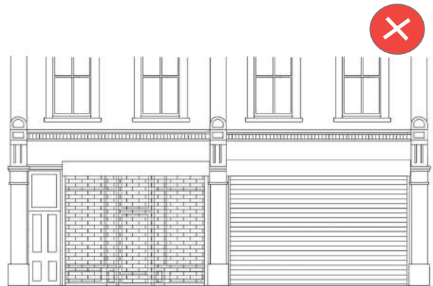
Picture 68. External Roller shutters are not appropriate.
